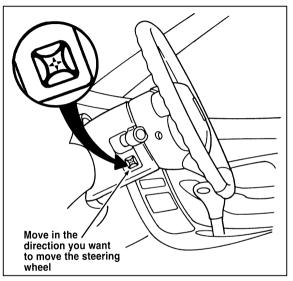
The lever to tilt the steering wheel
